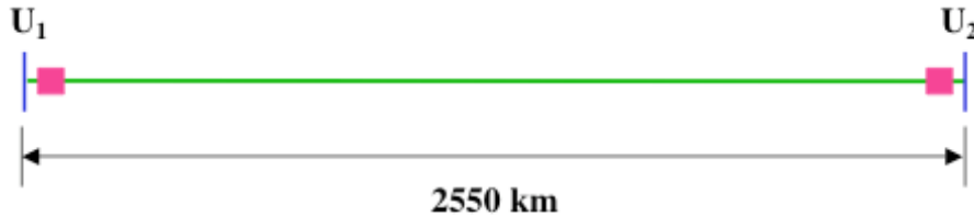
Fig. 8 – Schematic representation of a 1000 kV, 2550 km, three-phase line, with characteristic power P_c = 8.6 GW, without reactive compensation, switched from one extremity (all the line). Sustained overvoltage in one terminal (opened) is 1.017 pu (referred to the other terminal voltage).
